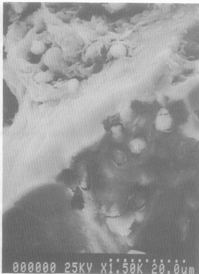
(b) Authigenic magnesite crystals growing in pits of surface of authigenic quartz crystal, suggesting that magnesite precipitation occurred after, or perhaps in conjunction with, corrosion of the quartz. (Scale bar=20 \mu\text{m} )
